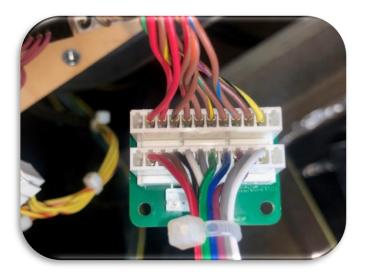
q) Take the pre-connected cable which is connected from the J2 socket of the Lamp Board Splitter board and route the unconnected end back to the CN8 socket of the Node Board 11 as shown below:
