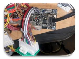
r) Connect the **unconnected end** of the Kiss Nano Topper cable that was inserted from above the playfield in **STEP 2(j)** and connect this into **J3 socket** of the Lamp Board Splitter board.
