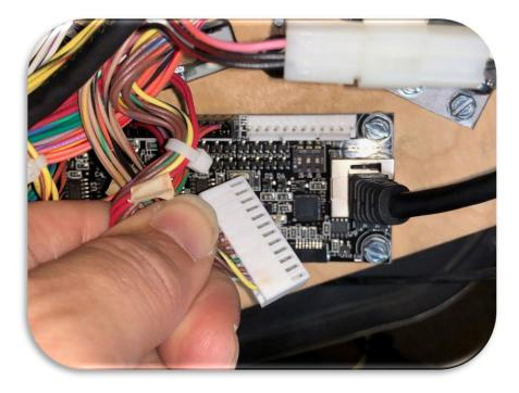
p) Connect the playfield CN8 cable into the <u>J1 socket</u> of the Lamp Board Splitter board as shown below. NOTE: The CN8 connector can <u>ONLY</u> be inserted one way as shown.
