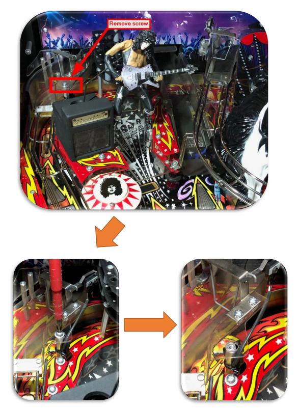
h) **PLEASE NOTE:** Place the metal screw and washer aside in a safe place as you will need this to attach the Kiss Target Nano Topper to the aluminium metal hex spacer later.
