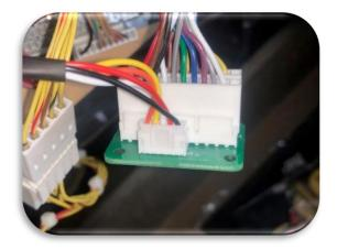
s) Using the supplied white cable tie, tie the cables from Lamp Board Splitter board to an existing fixed wiring loom securely as show below:
